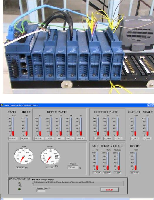
Figure 6. a) CFP2000 acquisition system with the acquisition and signal processing modules, b) screen of the code constructed with LabView 8.0 for control and acquisition.
